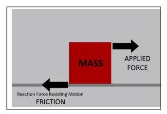
The image provided by VEX Robotics Design System illustrates the opposing relationship between an object's force and friction.
